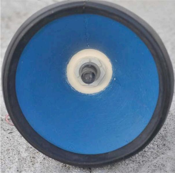
If the hydrophone is rigidly bonded to the body of the directional unit, it will be very sensitive to handling noise and water noise. Make a polystyrene collar to fit snugly over the hydrophone, and shape the outside to fit snugly into the bush inside the cone. Gently push into place inside the bush, then push the hydrophone through (from the rear). Then seal with a smear of Silicone RTV inside cone and inside the junction box.
