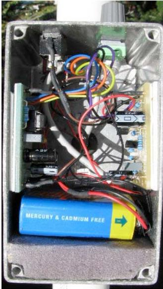
We house these boards, with a switched 9v battery, headphone socket and volume control (the 10k variable pot on the output of the champ), in an aluminium box.
