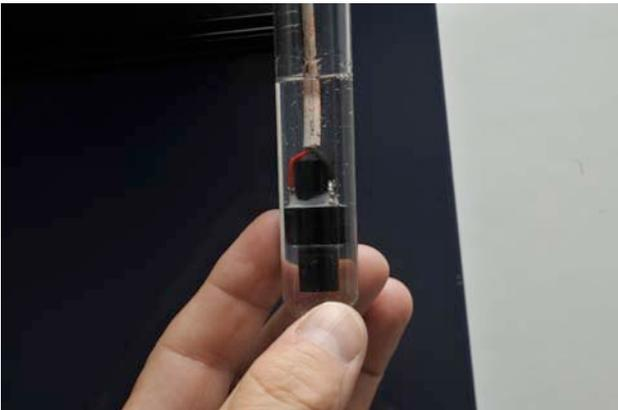
Pour 15 grms into the test tube, then insert the hydrophone element and coax. Work it up and down a bit to dispel air bubbles. Top up if necessary – the potting compound should completely cover the bare wires. Insert the foam spacer to ensure the wire exits from the middle of the moulding, not one side, and push down until just above the level of the potting compound. Tape top of test tube to cable and hang vertically for potting compound to go off.
