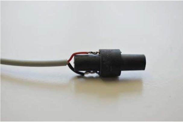
Solder the coax to the pins of the hydrophone element, so the shield goes to one pin and the core to the other. Make sure the two cannot short. Snip off the two pins on the other side. Abrade the outer jacket of the coax with sandpaper so that the potting compound will stick to it. Straighten the coax so that it and the element are as straight as possible.
